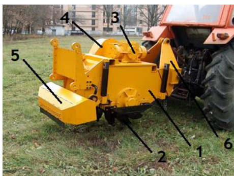
Fig. 3. Soil tillage mechanism prior to planting: 1 – casing; 2 – rotor; 3 – reducer; 4 – intermediate transmission; 5 – compactor; 6 – coupling triangle
