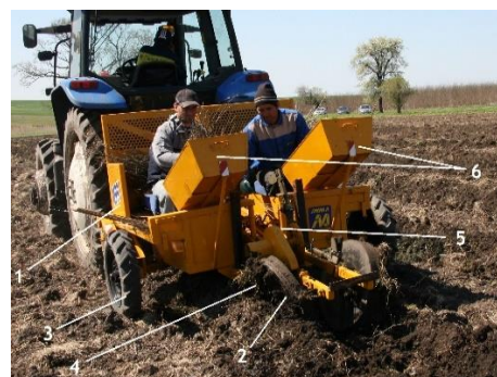
Fig. 4. Mechanism for planting forest saplings: 1 – frame; 2 – planting mechanism; 3 – transport train; 4 – watering pipe; 5 – mechanism for holding forest seedlings; 6 – seedling boxes
