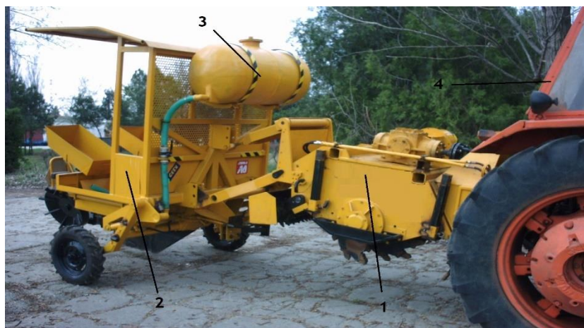
Fig. 1. Experimental installation design for planting forest saplings on difficult and desertified lands: 1 – soil processing equipment; 2 – seedling planting equipment; 3 – seedling irrigation equipment; 4 – agricultural tractor
